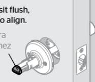
**D** Tip: Pull lever slightly away from door to see where screws insert.
