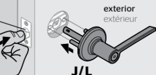
**⚠ IMPORTANT:** If installing a passage lock on an entry door, make sure the lever with the screw holes is on the interior side of the door.
