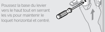
**F** Install interior lever and tighten pre-installed set screw.
