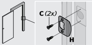
**B** Close door and test latch operation. If latch is loose in the strike, adjust strike tab so it grips the latch bolt better when the door is closed.
