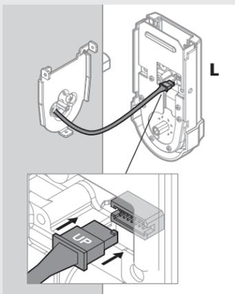
**E** Lay cable flat against the interior housing.
