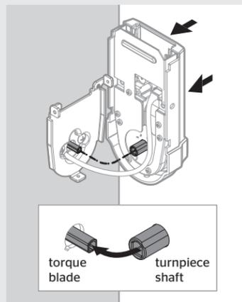
**G** Secure interior assembly with supplied screws.
