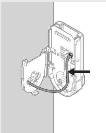
**F** Push turnpiece shaft onto torque blade.
